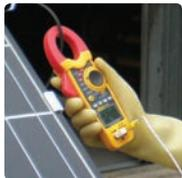
The SL200 Solar PV test kit includes the SL101 - Solar Irradiance Meter and the DL6402 - AC/DC current clamp meter packaged in a soft compact carry case.
